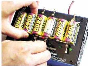
Install battery pack as shown
