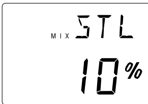
Steering-to-Auxiliary Channel Mixing Adjustment
