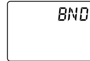
5. With the steering wheel and the throttle trigger in their desired failsafe positions, press the INCREASE and DECREASE buttons at the same time to enter bind mode. "BND" will flash when in bind mode.
